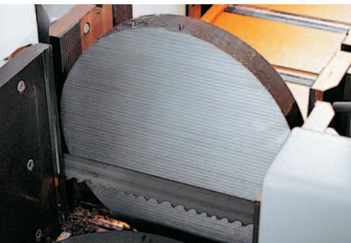
Less scrap, more profit: minimal rest piece length 35 mm, 50 mm for KASTOtec A7 in automatic operation.
