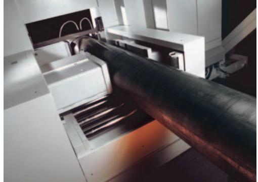
Save material transport for forged pieces with hydraulic horizontal infeed clamping device with pulling down clamping jaw.
