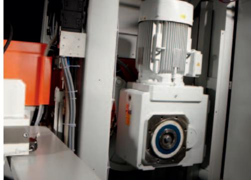
Strong and sensitive: frequency regulated helical-bevel motor directly at the drive wheel with concentric bearings.
