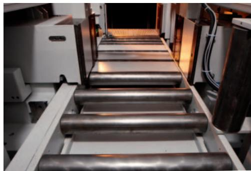
The continuous integrated machine roller conveyor simplifies material handling and transportation of short remnants.
